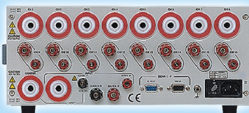
HSB-001-1 Rear Panel ( 8ch HV + 8CH GB )
